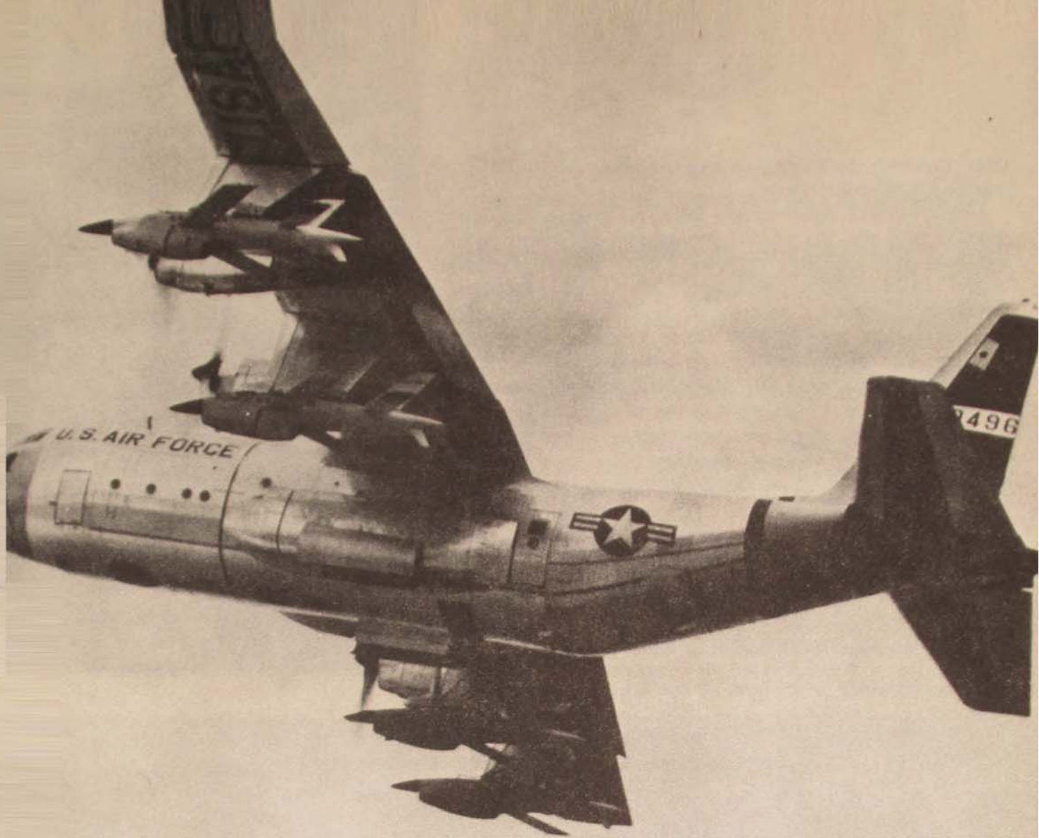
Aerial launch from a C-130 made dual launches possible. . . . Hughes Falcon missiles are loaded on an F-106 for a firing mission against the elusive drone target.
