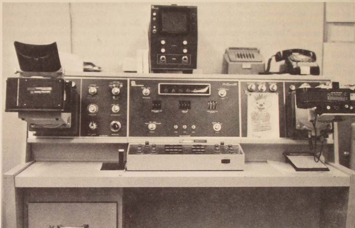
A gamma scintillation camera, one of the instruments used to obtain organ scans and perform dynamic studies of blood flow . . . Delineation of an abscess produced experimentally in a rabbit
