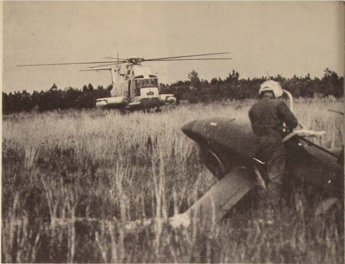
After landing safely on terra firma, the Firebee awaits pickup by a recovery helicopter.
